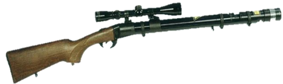
Figure 1 Laser rifle as used in ref. [1]. The Desman ® laser (model FL R 005) holds a 632.8 nm helium-neon laser with an output of 5 mW. Beam diameter at the exit is 12 mm and divergence is 0.3 mrad. It is labelled as Class 3B. (source: www.desman.fr )
